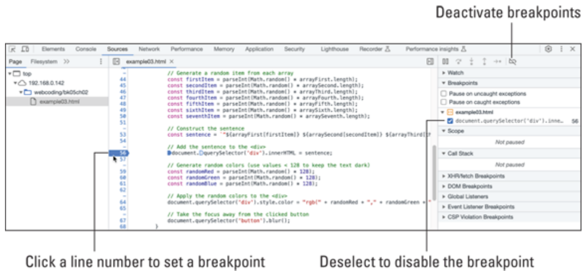
FIGURE 2-5: In the browser’s debugging tool, click a line number to set a breakpoint on that statement.
