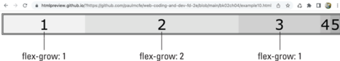
FIGURE 4-10: Items 1 and 3 get 25 percent of the container's empty space, whereas item 2 gets 50 percent.
