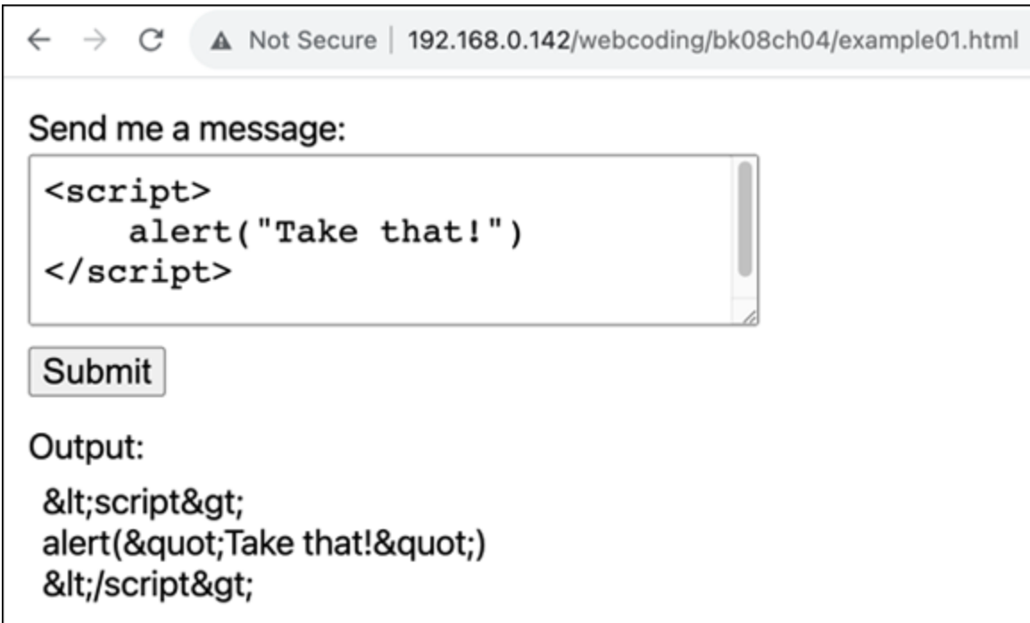
FIGURE 4-1: When this form is submitted, the JavaScript code in the text area gets sanitized.
