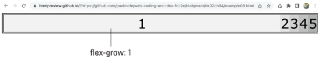
FIGURE 4-8: With flex-grow: 1 , an item grows until the container has no more empty space.
