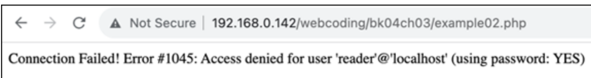
FIGURE 3-1: An example of an error number and message generated by the MySQLi object.
