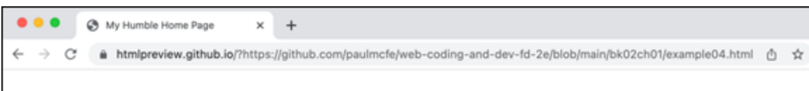
FIGURE 1-4: The text you insert into the <title> tag shows up in the browser tab.
