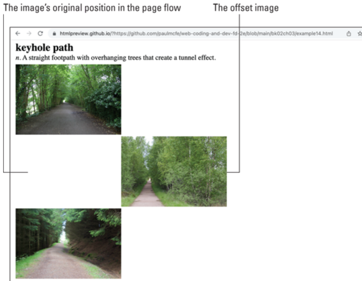
FIGURE 3-14: The middle image uses relative positioning to shift from the left, but its place in the page flow remains.
