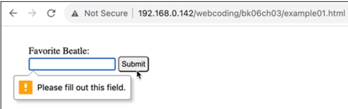
FIGURE 3-1: Add the required attribute to a form field to ensure that the field gets filled in.
